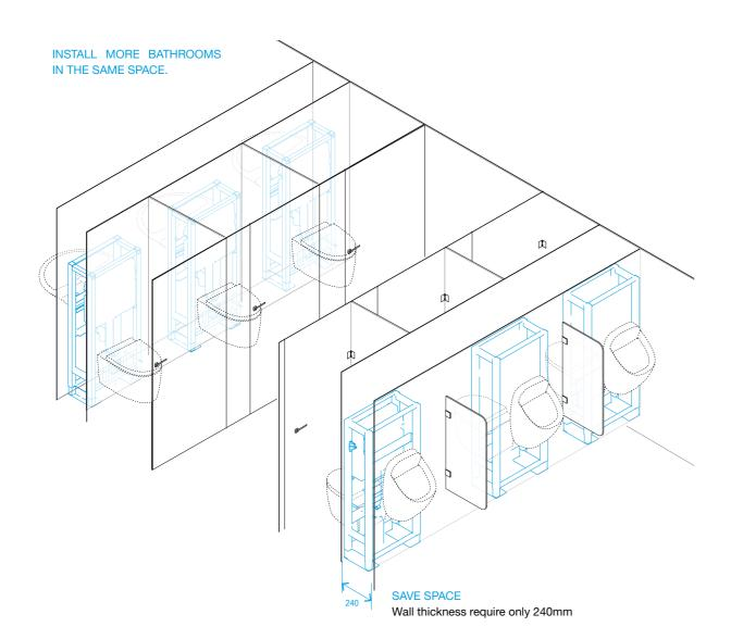
Independently of the bathroom, this product allows to place in one side a toilet and on the other side, a urinal or a washbasin, according to the acquisition of the kits and by sharing the same waste pipe connection, thanks to the evacuation pipe in Y shape. It is prepared to be fix to the floor suitable for plasterboard wall in technical frame.
